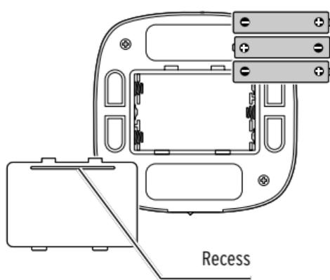
2. Use the recess in the battery compartment cover to gently pry the cover up and off.
