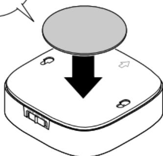
2. Remove the protective film from the back of the adhesive pad.
