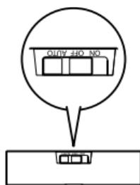
**ON** Slide the switch to **ON** to switch the light on permanently.
