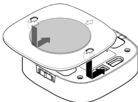
5. Reaffix the wall bracket by placing it on the back of the light and sliding it sideways (as illustrated). You must feel it click into place.
