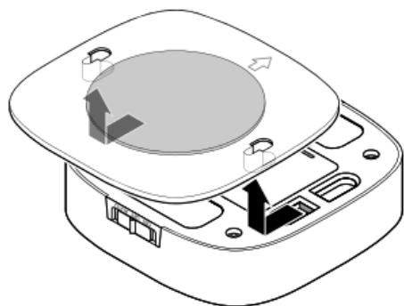
1. Remove the wall bracket on the back by pushing it to the side (as illustrated).
